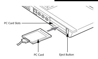
Figure 4-6. Installing/Removing PC Cards
